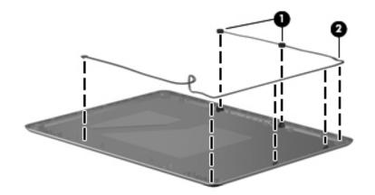
Reverse this procedure to install the microphone.
